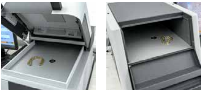
Easy sample positioning thanks to bottom up measuring direction and spacious measuring chamber
